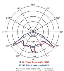
CO Plane beam angle (50%):123.0(DEG) C90 Plane beam angle (50%):124.8(DEG)
